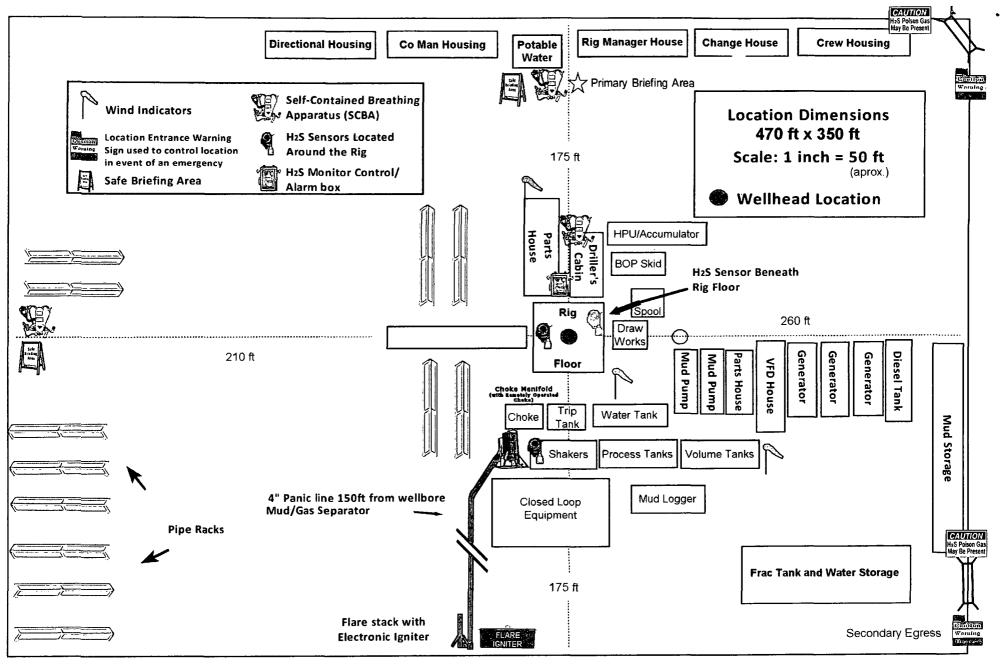
N Prevailing Wind Direction S, SW Devon Energy - Well Pad Rig Location Layout Safety Equipment Location
