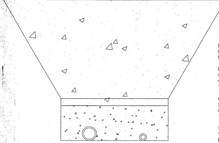
BACKFILL DIRT TO BE AS FREE OF ROCKS AND LARGE PARTICLES AS POSSIBLE
