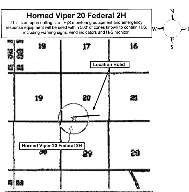
Assumed 100 ppm 3000' ( 100 ppm H2S concentration shall trigger activation of this plan.
