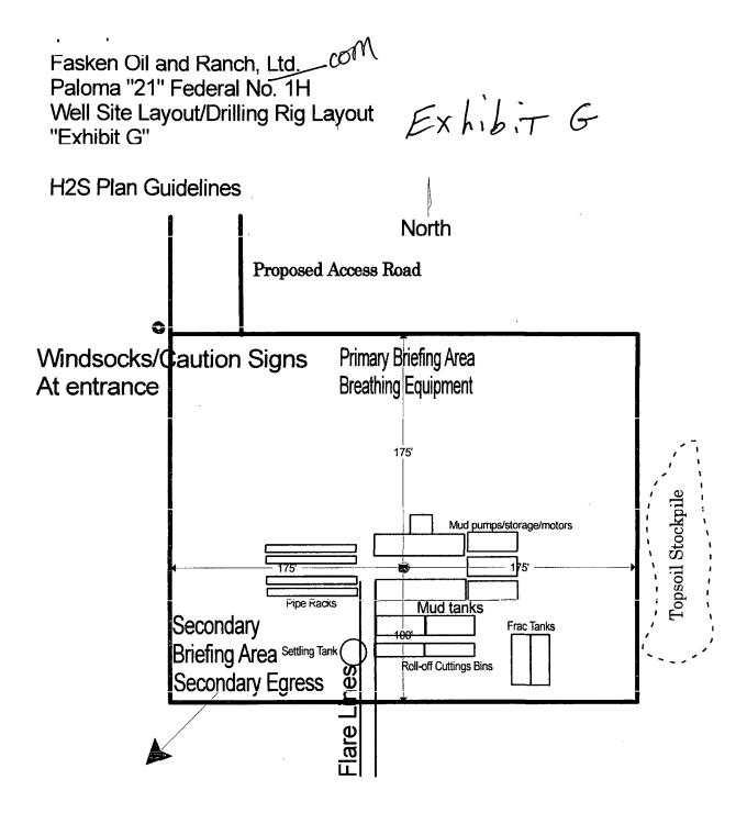
Alarms will be placed on the mud tanks, at the shale shaker, and on the rig floor. Windsocks will also be present on the top of the substructure and near the mud tanks.
