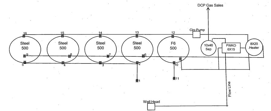
Production Phase: Valves: #1,2,3,4 5 Closed Valve: #10 Open Valves: #6,7,8 or 9 Open Valves: #13,14,15 or 16 Open
