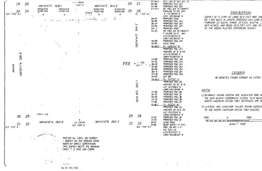
SURVEY OF A STRIP OF LAND 50 D FEET WDE AND 6864.5 FEET OR 1 300 MILES IN LENGTH CROSSING USA LAND IN SECTION 29. TOWNSHIP 23 SOUTH, RANGE 33 EAST, N.M.P.M., LEA COUNTY, NEW MEXICO. AND BEING 25 0 FEET LEFT AND 25 0 FEET RIGHT OF THE ABOVE PLATTED CENTERLINE SURVEY
