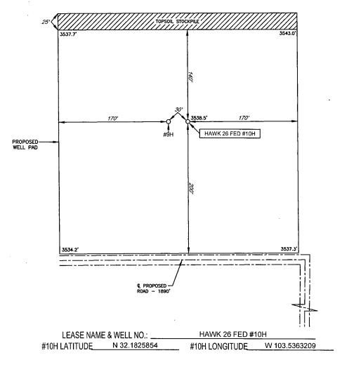
ALL BEARINGS, DISTANCES, AND COORDINATE VALUES CONTAINED HEREON ARE GRID BASED UPON THE NEW MEXICO STATE PLANE COORDINATE SYSTEM, EAST ZONE OF THE NORTH AMERICAN DATUM 1927, U.S. SURVEY FEET
