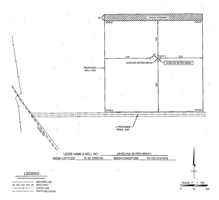
ALL BEARINGS, DISTANCES, AND COORDINATE VALUES CONTAINED HEREON ARE GRID BASED UPON THE NEW MEXICO STATE PLANE COORDINATE SYSTEM, EAST ZONE OF THE NORTH AMERICAN DATUM 1927, U.S. SURVEY FEET
