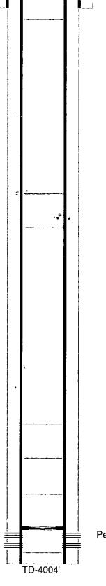
7-7/8" hole @ 4004' 5-1/2" csg @ 4004' w/ 1175sx-TOC-Surf-Circ
