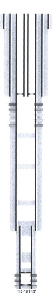
17-1/2" hole @ 772' 13-3/8" csg @ 772' w/ 915sx-TOC-Surf-Circ
