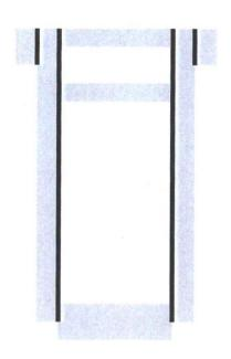
18-1/2" hole @ 352' 16" csg @ 352' w/ 470sx-TOC-Surf-Circ
