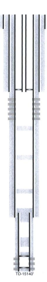
17-1/2" hole @ 772' 13-3/8" csg @ 772' w/ 915sx-TOC-Surf-Circ
