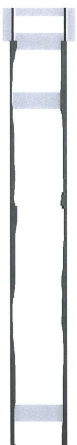
11" hole @ 388' 8-5/8" csg @ 388' w/ 300sx-TOC-Surf-Circ
