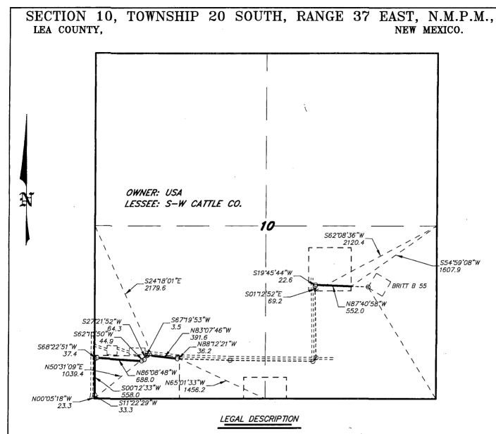
A STRIP OF LAND 30.0 FEET WIDE, LOCATED IN SECTION 10, TOWNSHIP 20 SOUTH, RANGE 37 EAST, N.M.P.M., LEA COUNTY, NEW MEXICO AND BEING 15.0 FEET LEFT AND RIGHT OF THE ABOVE PLATTED, CENTERLINE SURVEY.
