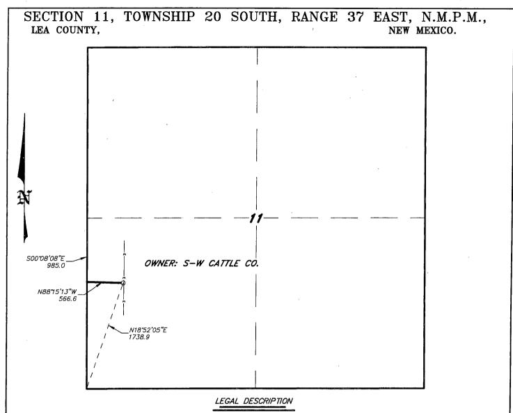
A STRIP OF LAND 30.0 FEET WIDE, LOCATED IN SECTION 11, TOWNSHIP 20 SOUTH, RANGE 37 EAST, N.M.P.M., LEA COUNTY, NEW MEXICO AND BEING 15.0 FEET LEFT AND RIGHT OF THE FOLLOWING DESCRIBED CENTERLINE SURVEY.
