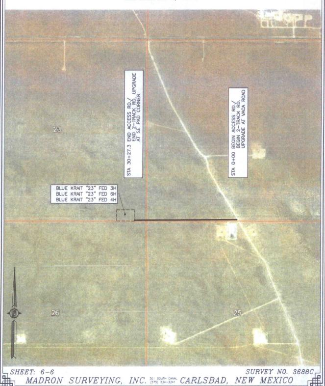
ELECTRIC LINE PLAT (400574E) ELECTRIC LINE TO CONNECT THE BLUE KRAIT "23" FED 1H, 10H, & 5H AND THE BLUE KRAIT "23" FED 3H, 6H, & 4H AND THE BLUE KRAIT "23" FED 2H AND THE BLUE KRAIT CENTRAL BATTERY DEVON ENERGY PRODUCTION COMPANY, L.P. CENTERLINE SURVEY OF AN ELECTRIC LINE CROSSING SECTION 24, TOWNSHIP 24 SOUTH, RANGE 33 EAST, N.M.P.M. LEA COUNTY, STATE OF NEW MEXICO OCTOBER 23, 2015 14 N89°40'03"E 2641.32 FT 13 N89°40'03"E 2641.32 FT RR SPIKE 24 19 23 #14 N00°27 S00°29'18"E SECTION LINE
