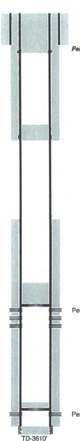
11" hole @ 301' 8-5/8" csg @ 301' w/ 325sx-TOC-Surf-Circ
