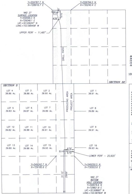
BOREPATH SHOWN HEREON IS BASED ON DIRECTIONAL SURVEY REPORT PROVIDED BY COG OPERATING, LLC FOR THE GOOSE STATE COM #2H SUPPLIED TO HARCROW SURVEYING, LLC ON JUNE 27, 2016
