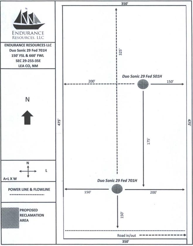
BLM has authorized multi-well (2 and 3 well pads) in lieu of single well pads, in conjunction with a centralized tank battery for the Duo Sonic 29 Fed productive wells. No reclamation is proposed at this time. Tank battery and wellsite will be constructed as needed by operations.
