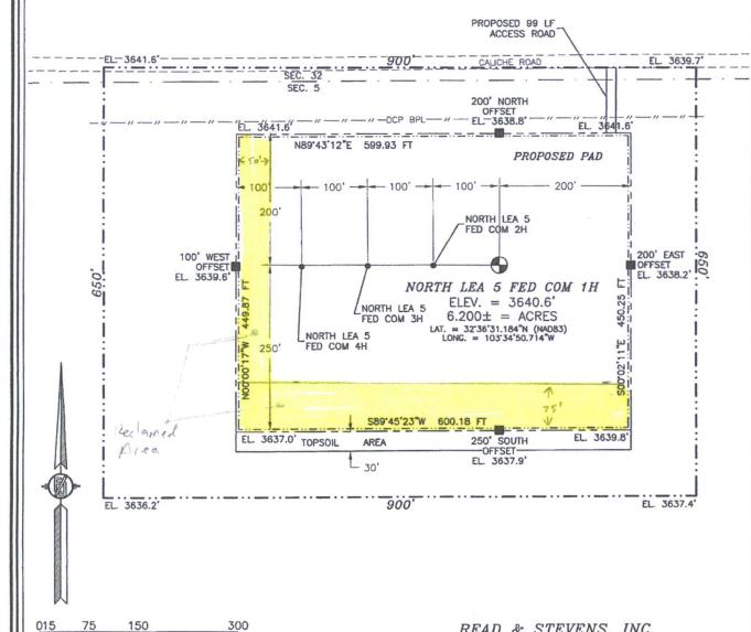
SCALE 1" 150 = DIRECTIONS TO LOCATION FROM MILE MARKER #78 ON HWY 62-180 GO WEST APPROX. 0.40 OF A MILE TO LEASE ROAD ON RIGHT (NORTH) TURN NORTH LEASE ROAD TURNS LEFT (WEST) GO APPROX. 0.40 OF A MILE, TURN LEFT GO SOUTH 99' TO THE NORTHEAST PAD CORNER FOR THIS LOCATION.
