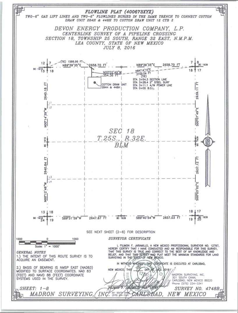
*FLOWLINE PLAT (400673XYZ)* TWO-6" GAS LIFT LINES AND TWO-6" FLOWLINES BURIED IN THE SAME TRENCH TO CONNECT COTTON DRAW UNIT 284H & 448H TO COTTON DRAW UNIT 12 CTB 2
