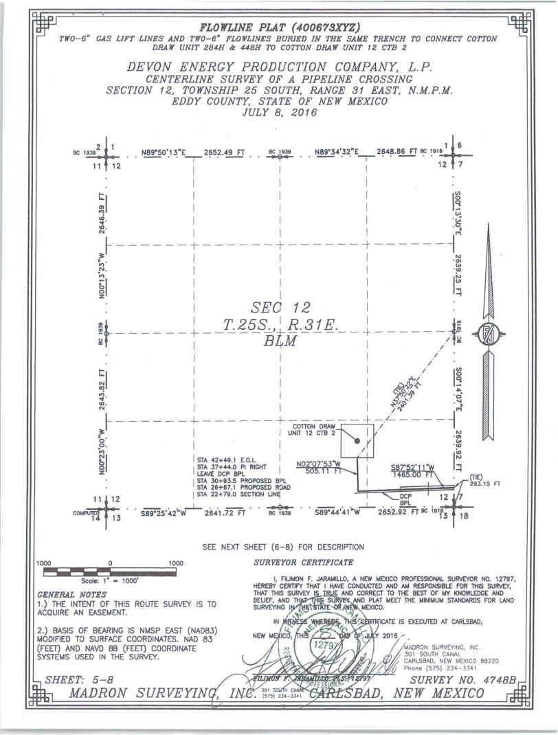
*FLOWLINE PLAT (400673XYZ)* TWO-6" CAS LIFT LINES AND TWO-6" FLOWLINES BURIED IN THE SAME TRENCH TO CONNECT COTTON DRAW UNIT 284H & 448H TO COTTON DRAW UNIT 12 CTB 2
