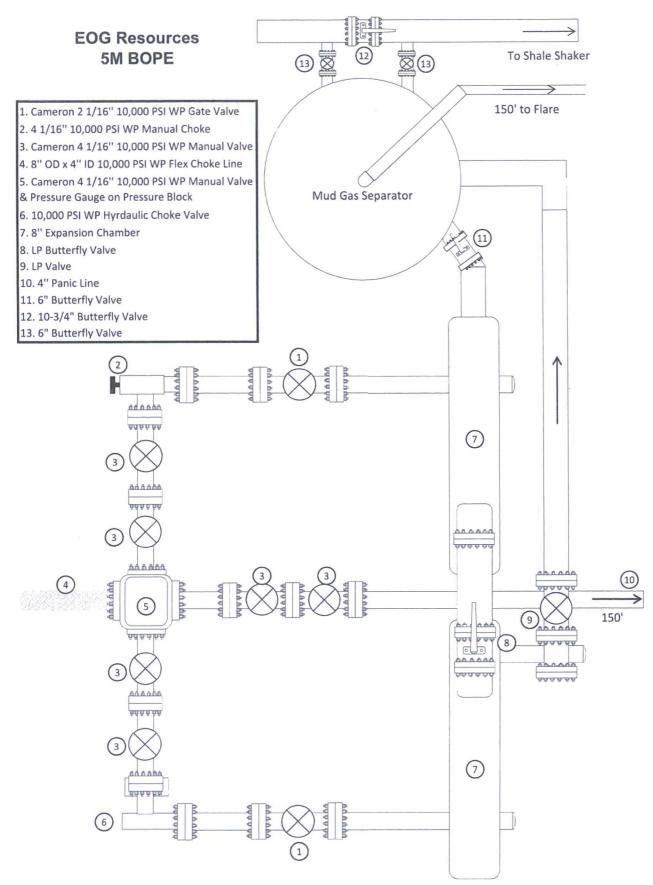
EOG 5M Choke Manifold Diagram (rev. 3/21/14)
