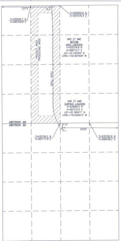
BOREPATH SHOWN HEREON IS BASED ON DIRECTIONAL SURVEY REPORT PROVIDED BY COG OPERATING, LLC FOR THE AZORES FEDERAL \$TH SUPPLIED TO HARCROW SURVEYING, LLC ON SEPTEMBER 22, 2016
