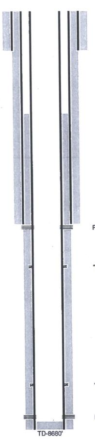
17-1/2" hole @ 805' 13-3/8" csg @ 805' w/ 945sx-TOC-Surf-Circ
