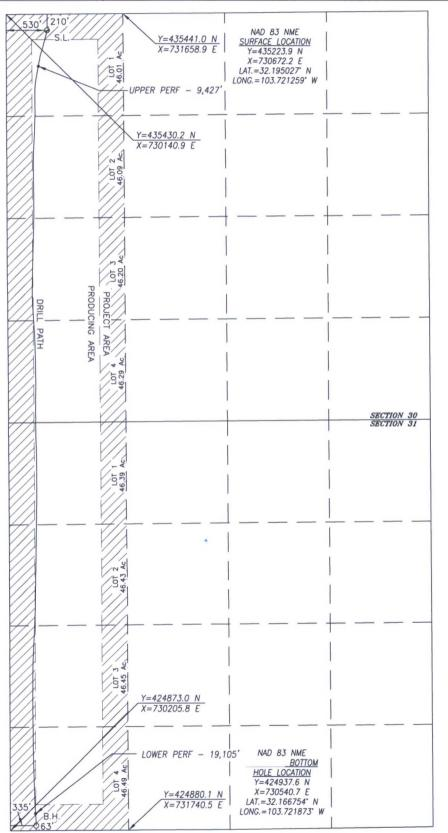
BOREPATH SHOWN HEREON IS BASED ON DIRECTIONAL SURVEY REPORT PROVIDED BY COG PRODUCTING, LLC. FOR THE WINDWARD FEDERAL SUPPLIED TO HARCROW SURVEYING, LLC ON OCTOBER 2, 2017.
