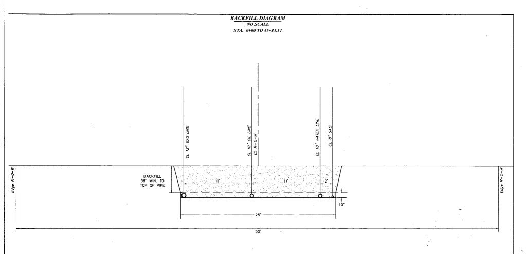
BACKFILL DIRT TO BE AS FREE OF ROCKS AND LARGE PARTICLES AS POSSIBLE
