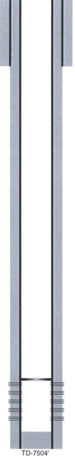
12-1/4" hole @ 1195' 8-5/8" csg @ 1195' w/ 620sx-TOC-Surf-Circ
