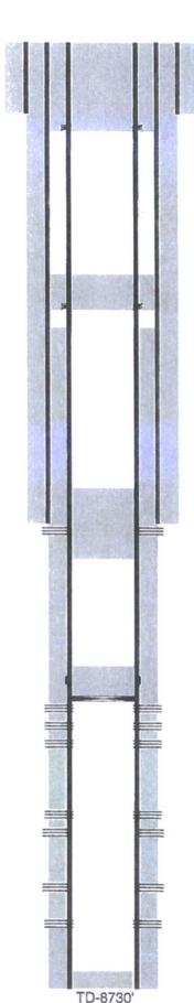
14-3/4" hole @ 805' / 10-3/4" csg @ 805' / w/ 780sx-TOC-Surf-Circ
