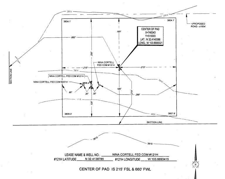
ALL BEARINGS, DISTANCES, AND COORDINATE VALUES CONTAINED HEREON ARE GRID BASED UPON THE NEW MEXICO COORDINATE SYSTEM OF 1983, EAST ZONE, U.S. SURVEY FEET
