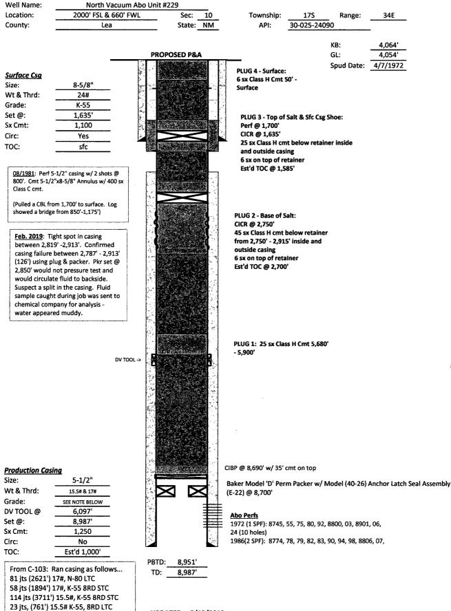
Cemented w/ 250 sx Class H neat. Opened DV Tool. Cemented w/ 1,000 sx Class C neat. No Circ. UPDATED: 2/13/2019
