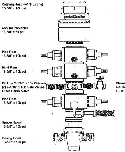
Choke Line 6" x 3" x 10k psi 4-1/16" x 10k psi Inner Manual Valve 4 - 1/16" x 10k psi Outer Remote HCR
