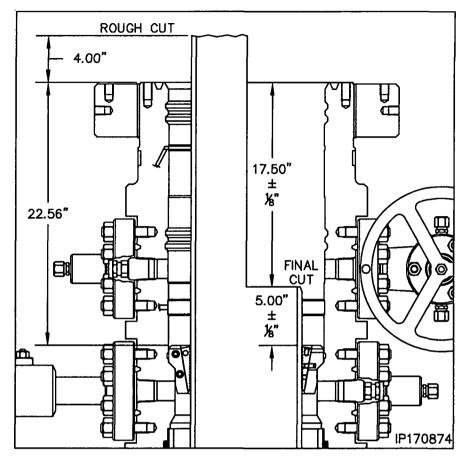
Note: There must not be any rough edges on the casing or the seals of the Packoff will be damaged.
