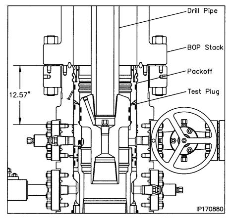
Remove as much fluid as possible from the BOP stack and the retrieve the test plug with a straight vertical lift.
