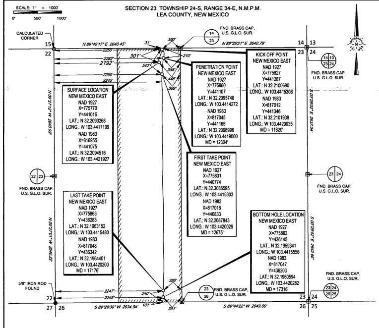
**BRAD LUMMIS COM 212H** LEASE NAME & WELL NO .: \_ SECTION 23 TWP 24-S RGE 34-E SURVEY N.M.P.M. ELEVATION \_\_3477' LEA NM COUNTY\_ \_\_\_ STATE. 301' FNL & 2192' FWL DESCRIPTION.
