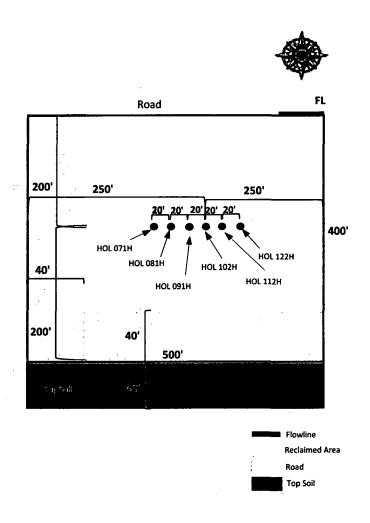
Holly Fed Com 26 36 05 071H SHL: 26S 36E 230' FNL 700' FWL Holly Fed Com 26 36 05 081H SHL: 26S 36E 230' FNL 720' FWL Holly Fed Com 26 36 05 091H SHL: 26S 36E 230' FNL 740' FWL Holly Fed Com 26 36 05 102H SHL: 26S 36E 230' FNL 760' FWL Holly Fed Com 26 36 05 112H SHL: 26S 36E 230' FNL 780' FWL Holly Fed Com 26 36 05 122H SHL: 26S 36E 230' FNL 800' FWL
