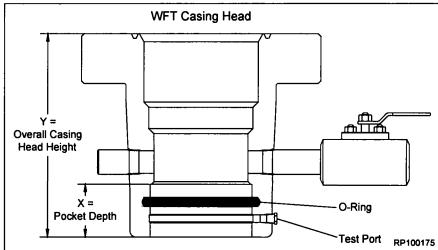
11. Final cut the surface casing at the correct elevation.
