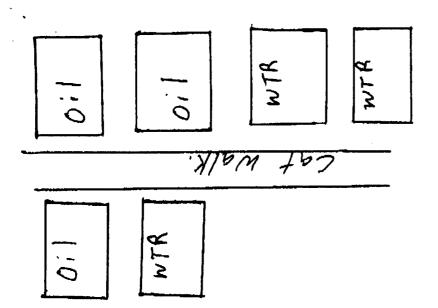
NOTE: 1-500-barrel oil tank & 1-500-barrel
