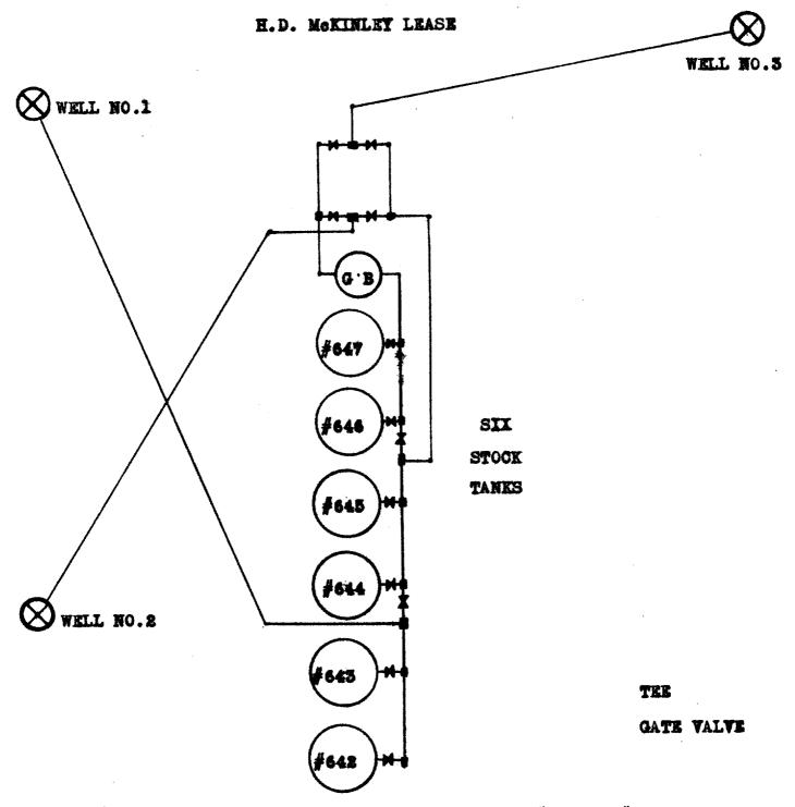
Well No.1 can be tested in either tank #642 or #645
