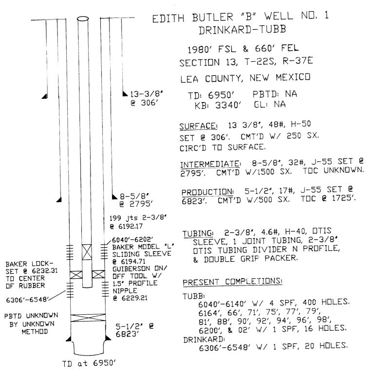
HISTORY: DRILLED IN 1947. COMPLETED OPENHOLE IN THE DRINKARD F/6823'-6950'. ADDED TUBB INTERVAL F/6040'-6140' IN 1957. ABANDONED OPENHOLE DRINKARD AND ADDED DRINKARD F/6306'-6548' IN 1974. ADDED PERFORATIONS IN TUBB F/6164'-6202'. ACIDIZED W/3000 GALS. FRAC'D ENTIRE TUBB W/50000 GALS 64000# 20/40 SD.
