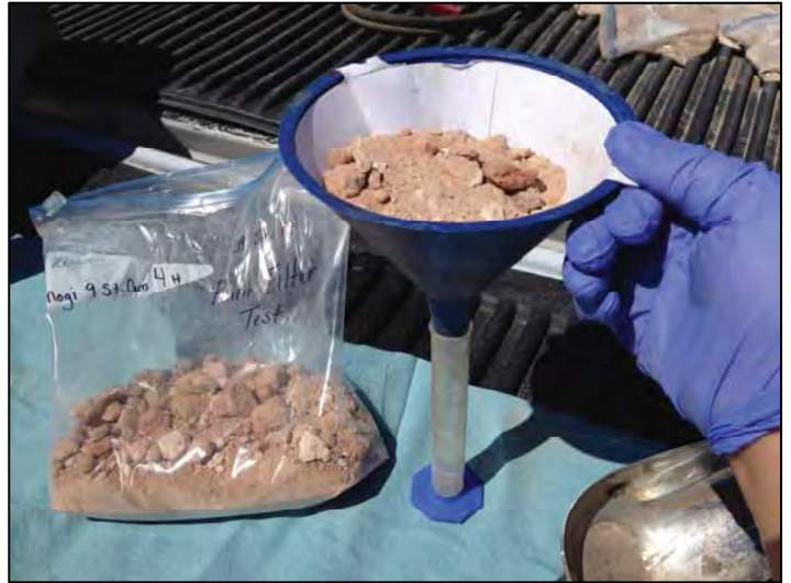
Paint Filter Test on Stabilized Cuttings 9/2/2014
