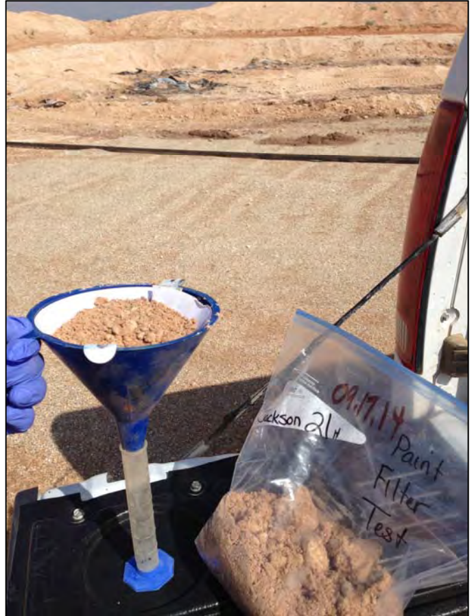
Paint filter test of stabilized cuttings 9/17/2014
