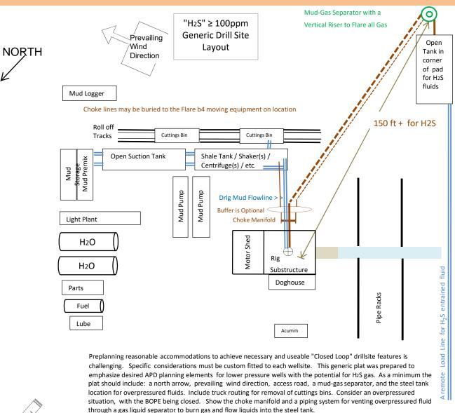
For a vertical gas vent or flare to be 150ft from the wellbore, the well needs to be centered in a square 250ft min on a side. To be 100ft from the wellbore, the well needs to be centered in a square 150ft min on a side.
