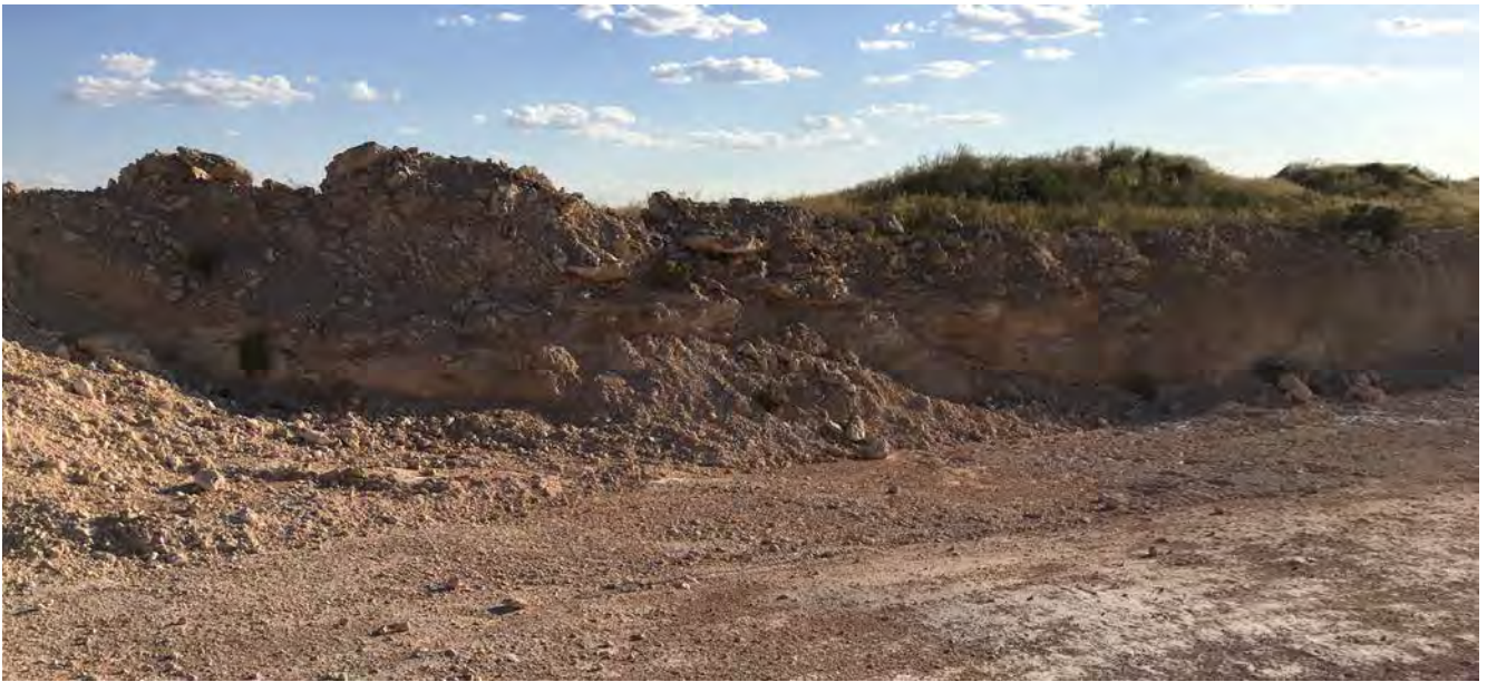
Caliche is present beneath the 2- to 5-foot veneer of stabilized dunes
