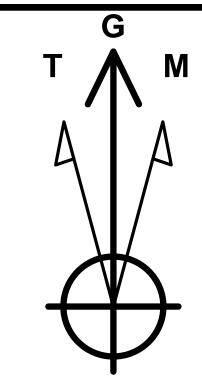
Azimuths to Grid North True North: -0.47° Magnetic North: 6.26°
