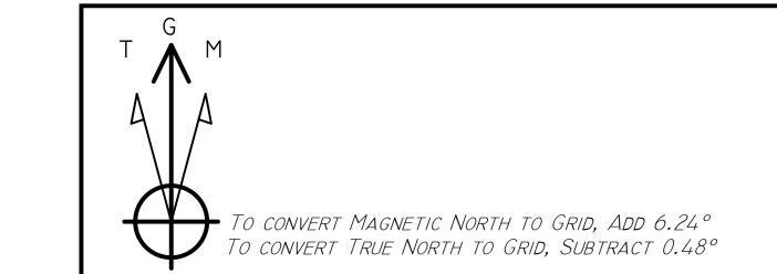
AZIMUTHS TO GRID NORTH TRUE NORTH: -0.48° MAGNETIC NORTH: 6.24° Magnetic Field STRENGTH: 47920.9SNT DIP ANGLE: 59.80° DATE: 4/9/2018 Model: HDGM
