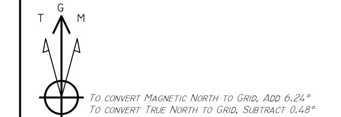
AZIMUTHS TO GRID NORTH TRUE NORTH: -0.48° Magnetic North: 6.24° Magnetic Field STRENGTH: 47919.6snT DIP ANGLE: 59.80° DATE: 4/9/2018 Model: HDGM
