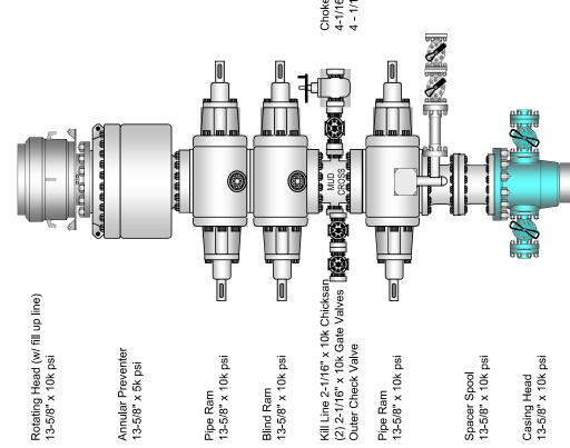
Choke Line 6" x 3" x 10k psi 4-1/16" x 10k psi Inner Manual Valve 4 - 1/16" x 10k psi Outer Remote HCR
