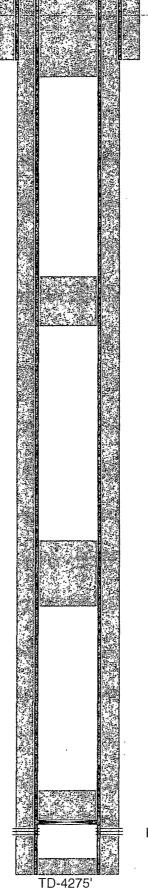
7-7/8" hole @ 4275' 5--1/2" csg @ 4266' w/ 1350sx-TOC-Surf-Circ
