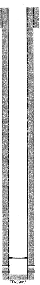
11" hole @ 314' 8-5/8" csg @ 314' w/ 200sx-TOC-Surf-Circ
