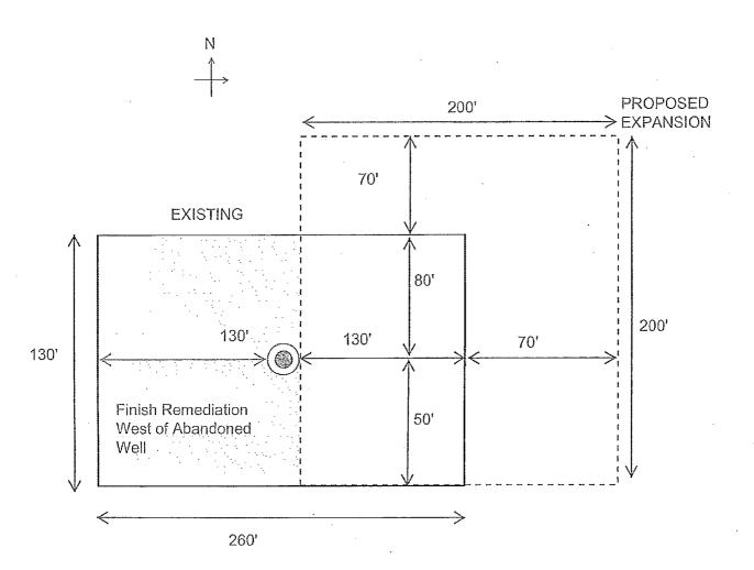
EXISTING PAD IS 130 FT (NORTH/SOUTH) AND 260 FT (EAST/WEST). EXPAND PAD 70 FT TO NORTH AND 70 FT TO EAST. NEW PAD DIMENSIONS WILL BE 200 FT X 200 FT. TANK DIAMETER IS 150 FT.
