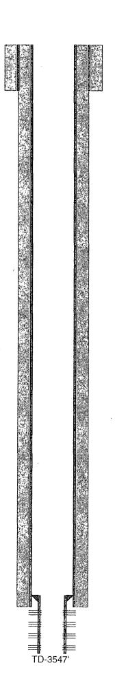
15" hole @ 302' 13-3/8" csg @ 302' w/ 175sx-TOC-Surf-Circ
