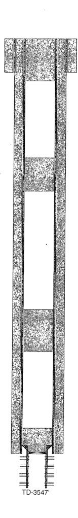
15" hole @ 302' 13-3/8" csg @ 302' w/ 175sx-TOC-Surf-Circ
