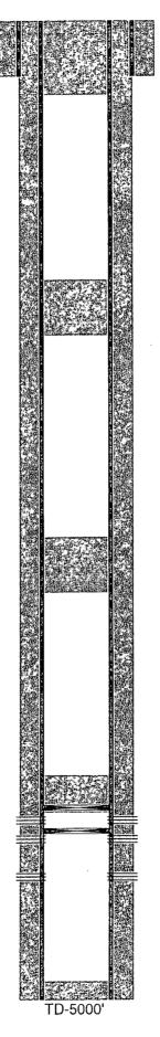
12-1/4" hole @ 352' 8-5/8" csg @ 352' w/ 350sx-TOC-Surf-Circ
