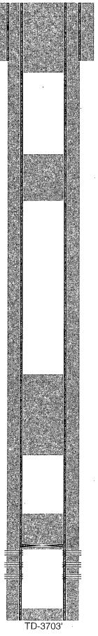
12-1/4" hole @ 376' 8-5/8" csg @ 376' w/ 315sx-TOC-Surf-Circ
