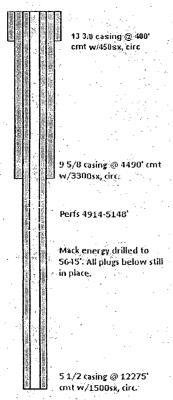
13 3/8 casing @ 400° cmt w/450sx, circ 9 5/8 casing @ 4490' cmt w/3300sx, circ. Proposed: Set CIBP @ 5080' w/ Perfs 4914-5148' 35' cmt cap. Mack energy drilled to S645'. All plugs below still in place. 5 1/2 casing @ 12275'
